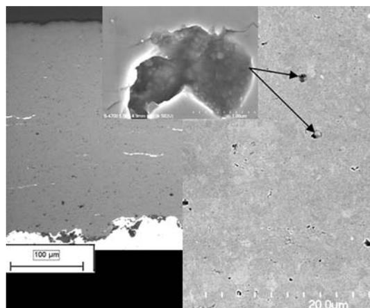
**Fig. 7** Cross-sectional view of n-TiO<sub>2</sub> coating deposited using a proprietary process: LOM (left); FE-SEM of coating (right) and porous particles (center)
