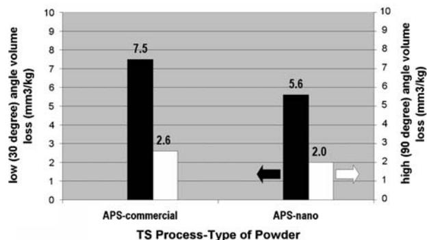
**Fig. 6** Slurry erosion volume loss at low and high impingement angles for commercial and nanostructured TiO<sub>2</sub> coatings applied via APS
