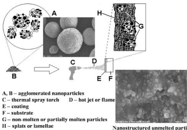
**Fig. 1** Generic schematic to thermal spraying of nanostructured ceramic coatings
