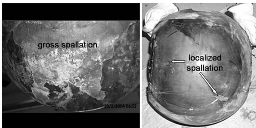
**Fig. 11** Photographs of the ball surfaces with Cr<sub>2</sub>O<sub>3</sub>-blend coating (left) and with n-TiO<sub>2</sub> coating (right) after same service exposure and conditions
