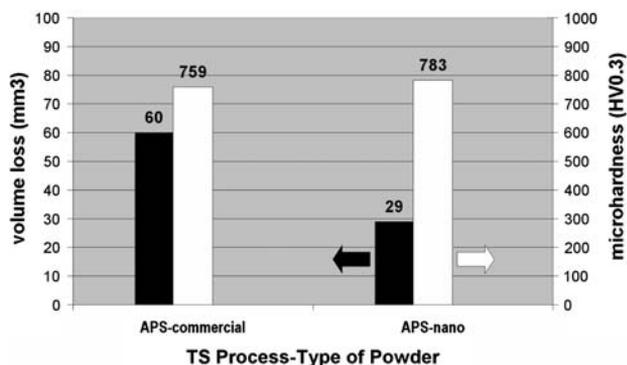
**Fig. 5** Abrasive wear volume loss and microhardness (HV300) of commercial and nanostructured TiO<sub>2</sub> coatings applied via APS
