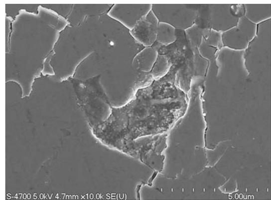
**Fig. 4** Field emission-SEM micrograph of cracks in porous nanostructured unmelted particles
