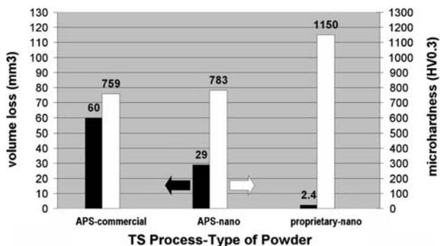
**Fig. 9** Abrasive wear volume loss and microhardness (HV300) of commercial and nanostructured TiO<sub>2</sub> coatings applied
