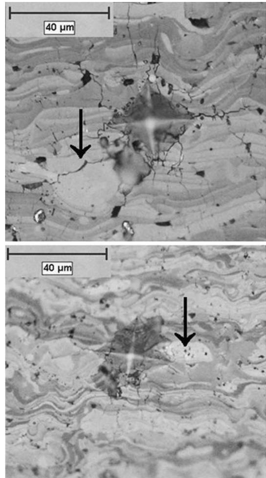
**Fig. 3** Micro-indentation crack pattern on commercial (top) and nanostructured (bottom) APS-applied TiO<sub>2</sub> coatings
