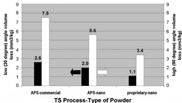
**Fig. 10** Slurry erosion volume loss at low- and high-angle impingement for commercial and nanostructured TiO<sub>2</sub> coatings
