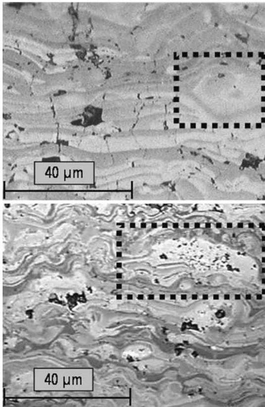
**Fig. 2** Cross-sectional view of APS TiO<sub>2</sub> Coatings: conventional (top) and nanostructured (bottom)
