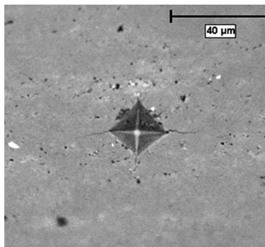
**Fig. 8** Micro-indentation crack pattern on n-TiO<sub>2</sub> deposited using a proprietary process
